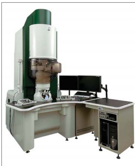
Fig.1 – Microscopul electronic JEM ARM 200F instalat la INCDFM
