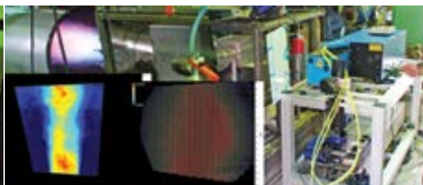
Laserometrie-LIF (Laser Induced Fluorescence)/PIV (Particle Image Velocimetry)
