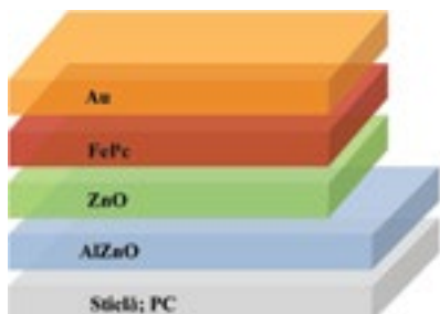
Figura 2. Arhitectura diodelor hibride organic/anorganic FePc/ZnO
