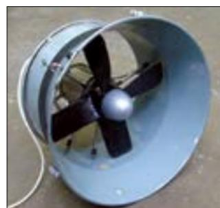
Microhidrogenerator electric intubat
